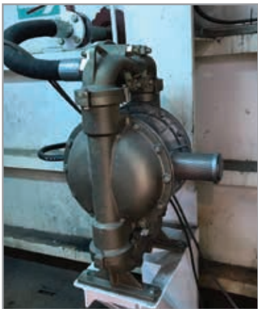
ASIA. Off-shore platform MISTRAL (DDM 200) pump for transferring water charged with oils during wastewater treatment phase.
