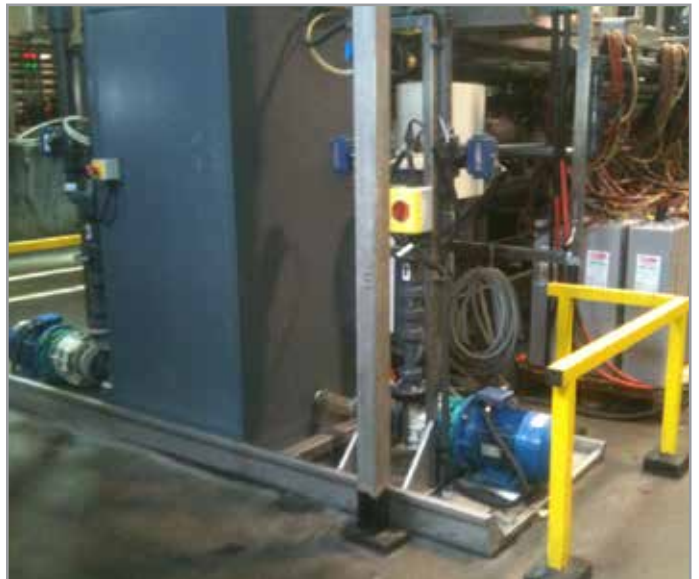
ITALY. Storage battery plant - ROUTE pumps for the circulation of acids into batteries.
