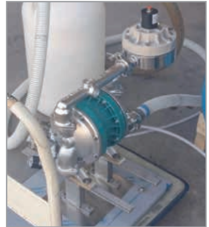
ITALY. Dairy industry ASTRAevo (DDE 160 AISI316L) pump with pulsation dampener.
