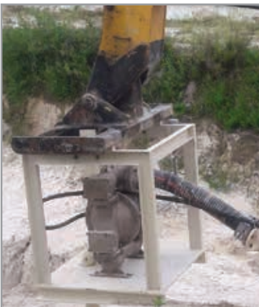
ITALY. Mineral extraction (silice) MISTRAL (DDM 400 AISI316L) pump for silice extraction.
