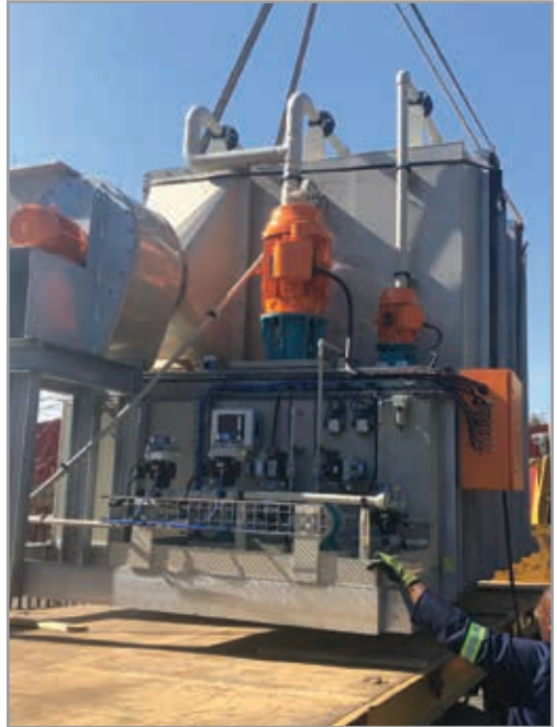
SOUTH AFRICA. Emergency chlorine fume scrubber K2 (KGK) for transferring wastewater containing chloride.
